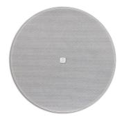
The Apart CM20DT is a 2-way 100V / 70V / 16 ohm built-in design ceiling loudspeaker. The loudspeaker has a 6  $\frac{1}{2}$ " woofer, a 1" coaxial tweeter and a high quality 100 / 70 volt loudspeaker line transformer with multiple power taps. CM20DT is the perfect choice for the distribution of microphone calls and background music. The mounting frame is made of high quality ABS. The steel grille is kept in place by strong magnets.
